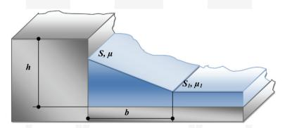
Fig. 1. Drifted snow load zone in the places of height discontinuity (according to codes of structural design)
