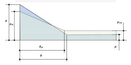
Fig. 2. Correction algorithm of design values of drifted snow load
