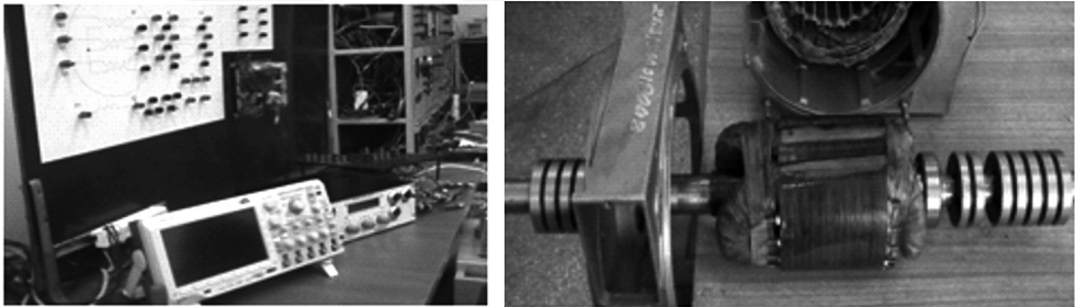
Fig. 9. Measurement set for investigation of the induced voltages in the 5 damping bars of the 5.5 kVA salient pole synchronous generator with the special construction of the rotor
