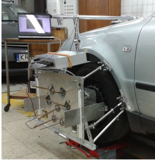
Fig. 4. An overview of the prototype measuring instrument attached to the car wheel
