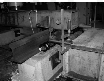
Fig. 3. Sample with forcing element and measuring system during vertical stiffness test
