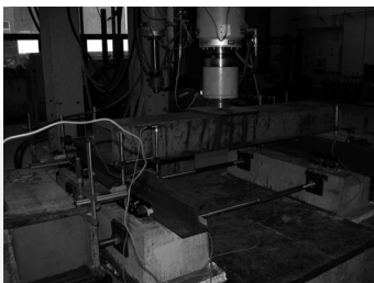
Fig. 2. LONGASF sample with ICOSTRUN 03 during stiffness tests [1]
