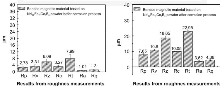
Fig. 3. Selected parameters of the surface profile for  $\text{Nd}_{12}\text{Fe}_{77}\text{Co}_5\text{B}_6$  bonded magnetic material (powder bonded with biopolymer): a) before corrosion test, b) before corrosion test
