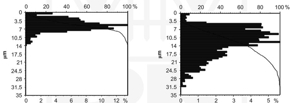
Fig. 4. Abbott curve and distribution of surface elevations for  $\text{Nd}_{12}\text{Fe}_{77}\text{Co}_5\text{B}_6$  bonded magnetic material (powder bonded with biopolymer): a) before corrosion test, b) after corrosion test
