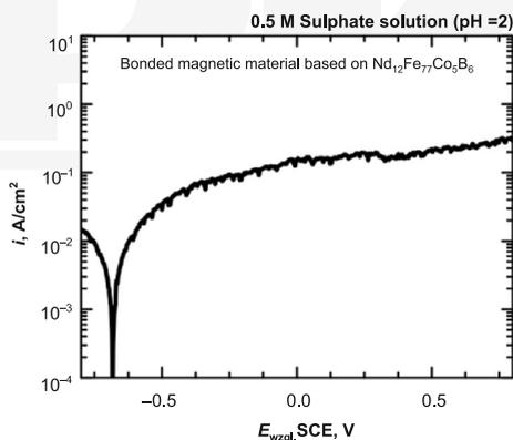
Fig. 1. The potentiokinetic polarization curves for samples obtained from  $\text{Nd}_{12}\text{Fe}_{77}\text{Co}_5\text{B}_6$  powder encapsulated with biopolymer measured in 0.5 M sulfate solution acidified to pH = 2 ( $10 \text{ mV}\cdot\text{s}^{-1}$ ,  $16 \text{ r}\cdot\text{s}^{-1}$ ,  $20^\circ\text{C}$ ) – powder consolidated with biopolymer
