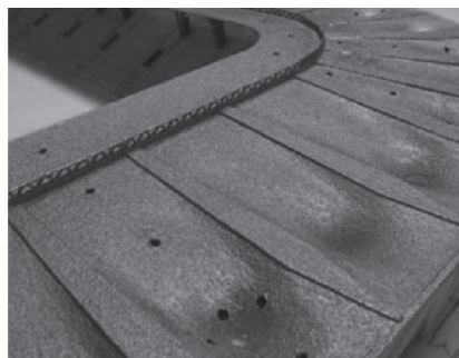
Fig. 3. a) stadium model with its immediate surroundings in the wind tunnel working section, b) a part of the stadium roof model with pressure taps
