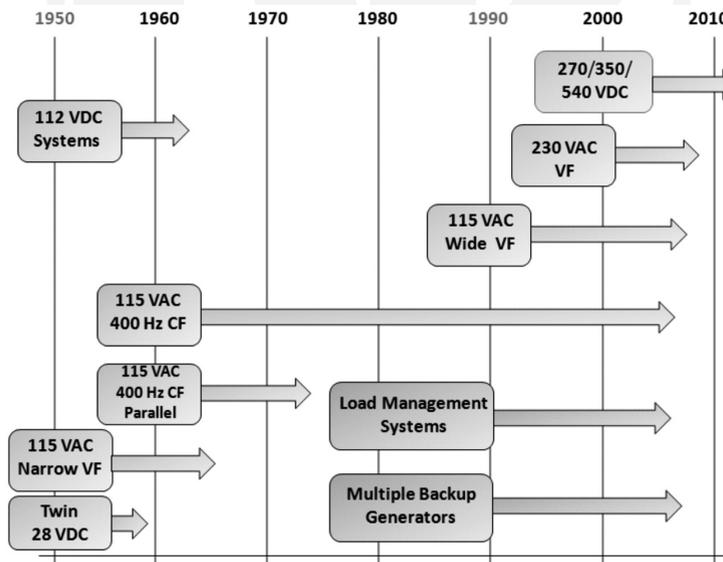
Fig. 1. Electro-energy Systems Evolution of Aircraft [4]
