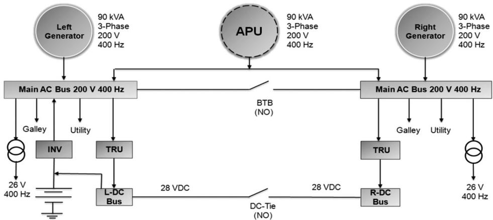
Fig. 4. Conventional B-767 Aircraft Power Distribution System [4, 6]
