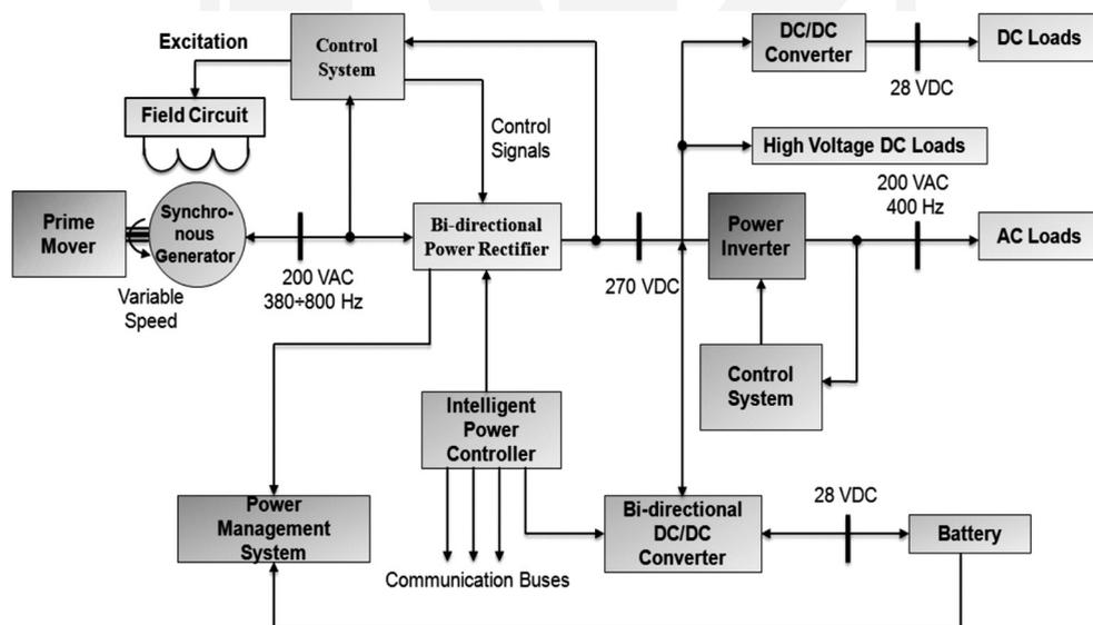
Fig. 5. More Electric Aircraft (MEA) Power Distribution System [6]
