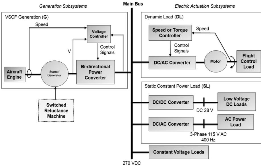
Fig. 6. 270 DC Power System for MEA [7]
