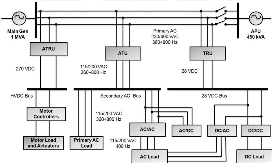
Fig. 7. B-787/A-380 Aircraft Power Distribution System [4, 7]
