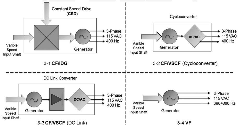
Fig. 3. Electric Power Generation Development of Civil Aircraft [4, 5]
