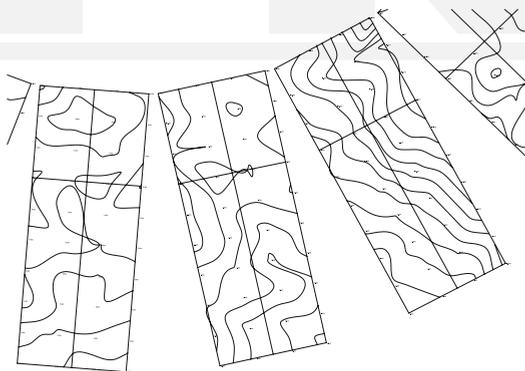
Fig. 8. Plate deformation isolines upon tensioning [4]
