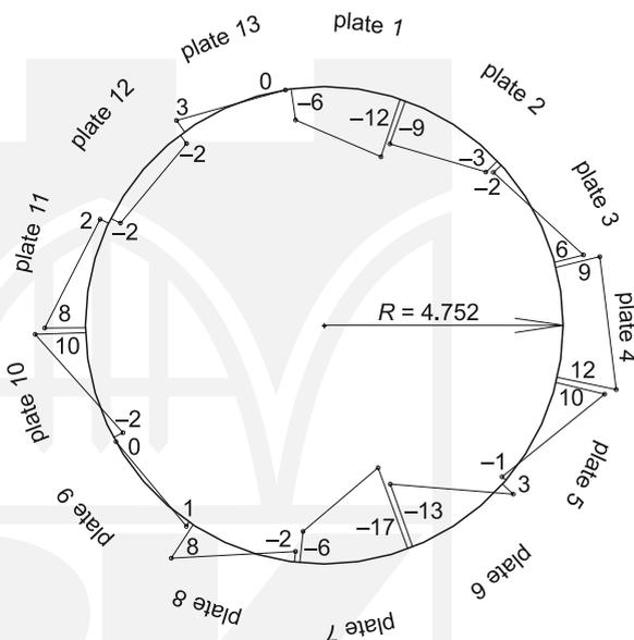
Fig. 7. Plate deflections from optimum location [3]
