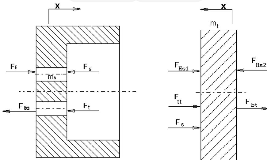
Fig. 4. Forces acting on the slider and piston controller
