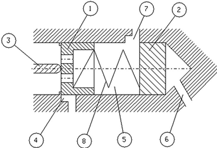
Fig. 3. Simplified schematic of the flow controller
