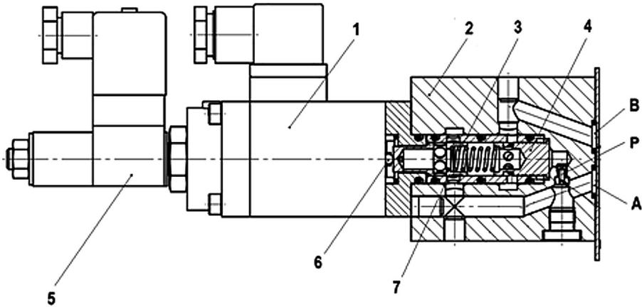
Fig. 1. Diagram of two-way proportional flow control
