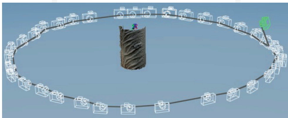
Fig. 4. Positions of the camera during a series of 35 photographs of the iced cable model
