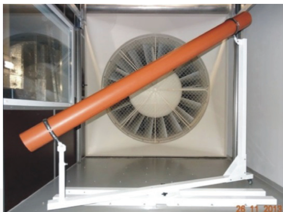
Fig. 2. View of the support of the cable model on the special frame placed in the climatic section of the wind tunnel
