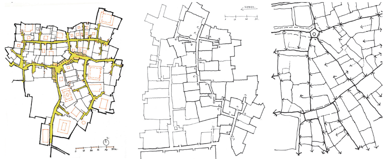
Fig.6. Left: Plan of the residential district of Mokhfiya in Fez, composed of several housing clusters extending around internal dead-end alleys or cul-de-sacs, source: Bianca, 2000, p.150. Centre: Plan of two residential clusters in Fez with a variety of self-contained courtyard houses, source: Bianca, 2000, p.83. Right: Part layout of Al-Adl section in Riyadh depicts the layout of an urban block, source: Talib, 1984, p.13.
