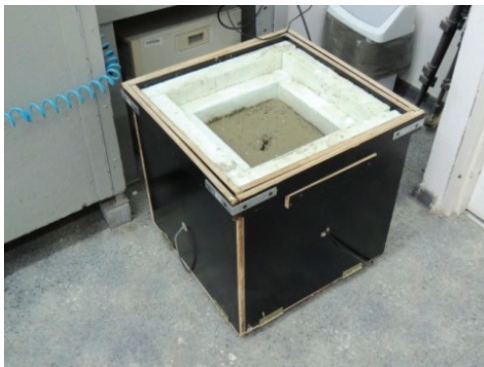
Fig. 3. Sample of fresh concrete with thermal insulation and the Vikasonic system as prepared for measurement
