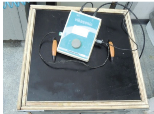
Fig. 3. Sample of fresh concrete with thermal insulation and the Vikasonic system as prepared for measurement
