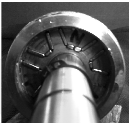
Fig. 4. Rotor of the physical model of the six-pole single-phase line start permanent magnet synchronous motor
