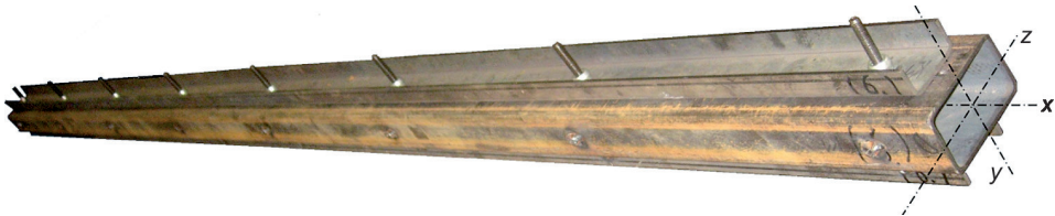
Fig. 16. Three-branched column foreseen for test (before installation of BOM fasteners)
