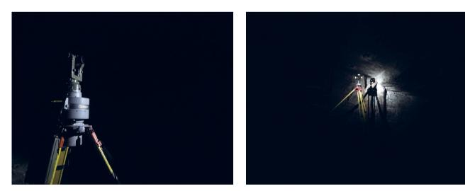
Fig. 2. Underground gyroscopic measurement (Gyromat 2000) and polygonisation, Crystal Grottoes in Salt Mine Wieliczka, authors' own archive
