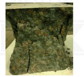
Fig. 4. Typical failure modes of SCC1
