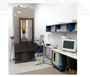
Fig. 2. MTS testing system for uniaxial compression tests
