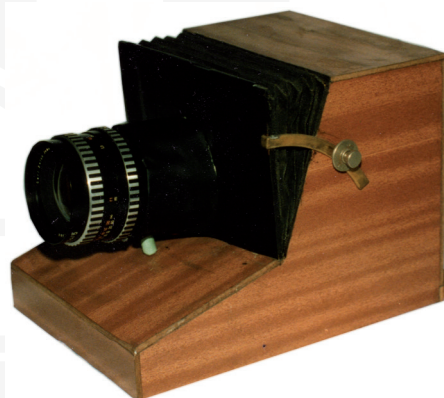
Ill. 4. A prototype of the optical device “Anamorphot” (project development: A. Zdziarski)
