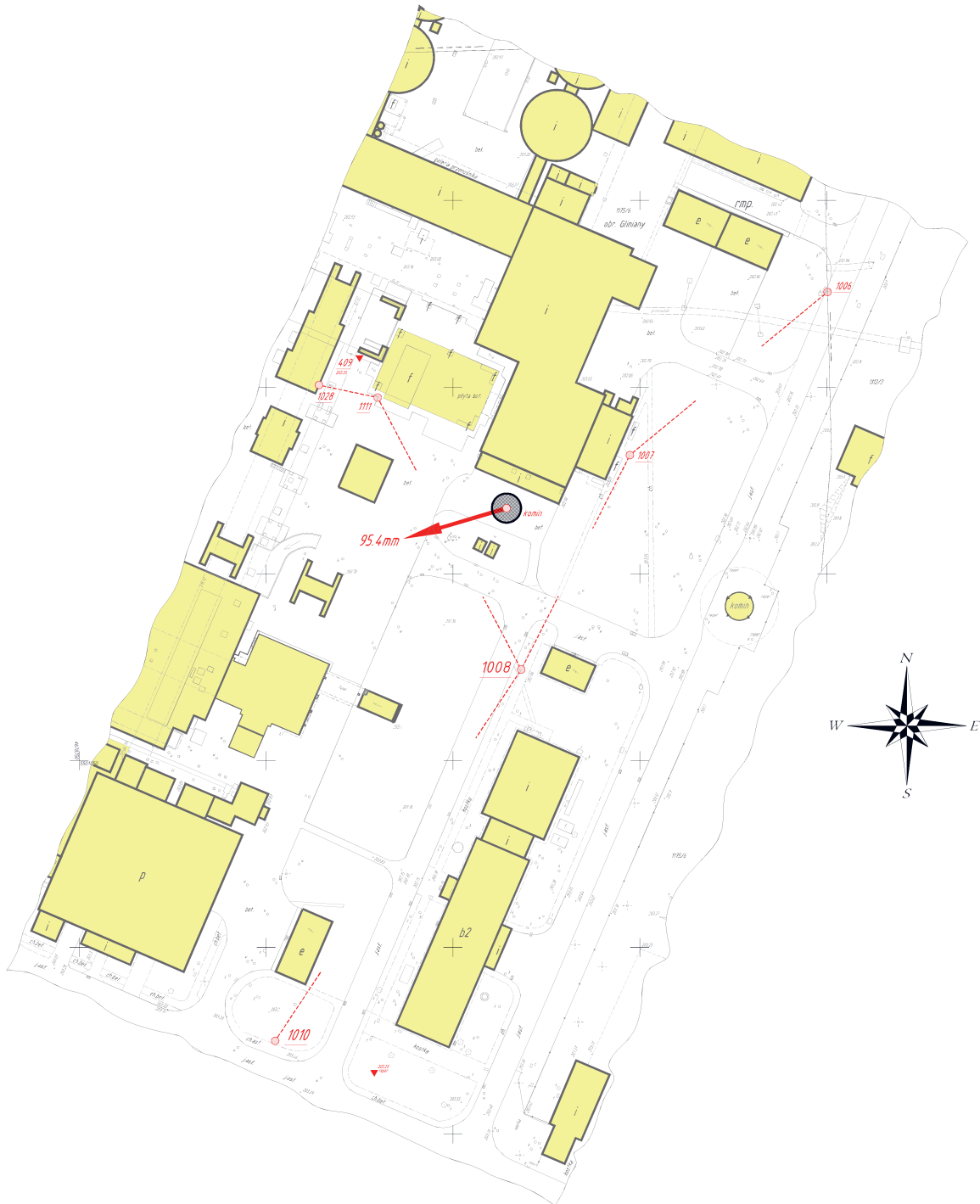
Fig. 3. Situation – altitude map of the industrial area in the vicinity of the inventoried industrial chimney of the Cement Plant „Ożarów” 1006, 1008, 1111 – measurement points; 1007, 1010, 1028 – situation reference points; 409 – altitude reference point. Distanced of measurement points from the measured chimney: 103.5m (point 1006); 43.4m (point 1008); 45.5m (point 1111).
