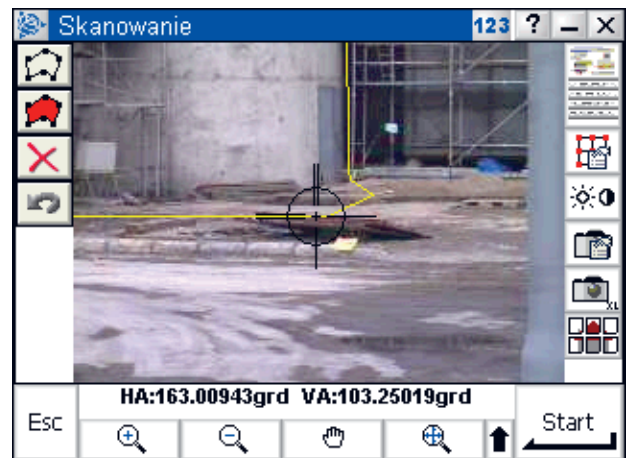
Fig. 1. The image from the camera of the total station with the marked fragment of the area where the chimney's base was scanned (interrupted yellow line)
