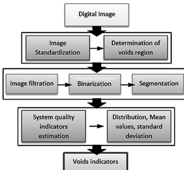
Fig. 1. The general scheme of the voids estimation and image analysis process
