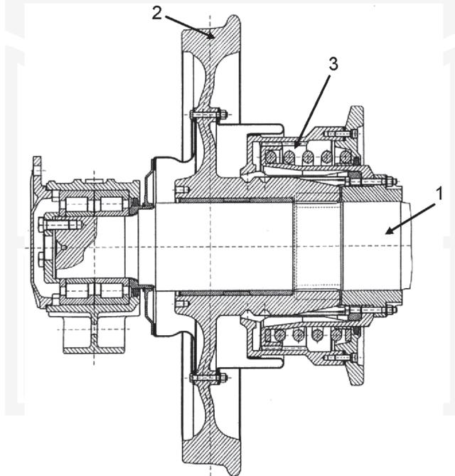
Fig. 1. Cross-section of wheel set with an automatic gauge change system [1]
