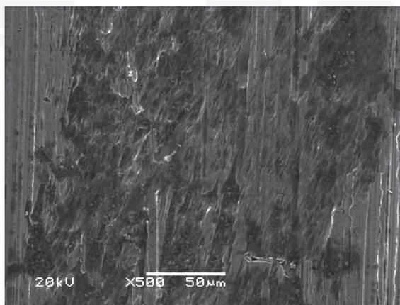
Fig. 6. Scanning picture of fretting damage on shaft seat – pits and material ridges in damage area and its oxidation, magn. 100× and 500×
