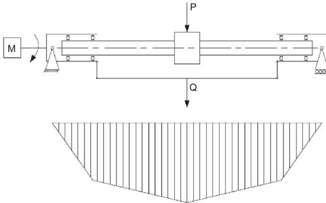
Fig. 3. Specimen loading and bending moment distribution
