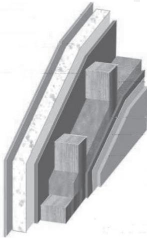
Ill. 1. Cross section of the frame wall [6]
