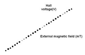
Fig. 3. Hall effect sensor characteristic
