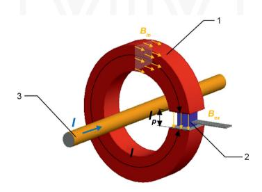
Fig. 1. Schematic diagram of current sensor: 1 - magnetic field concentrator, 2 - Hall sensor, 3 - wire under test
