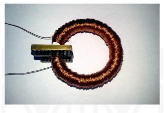
Fig. 4. Constructed DC current transformer
