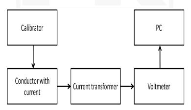
Fig. 5. Schematic of the test stand
