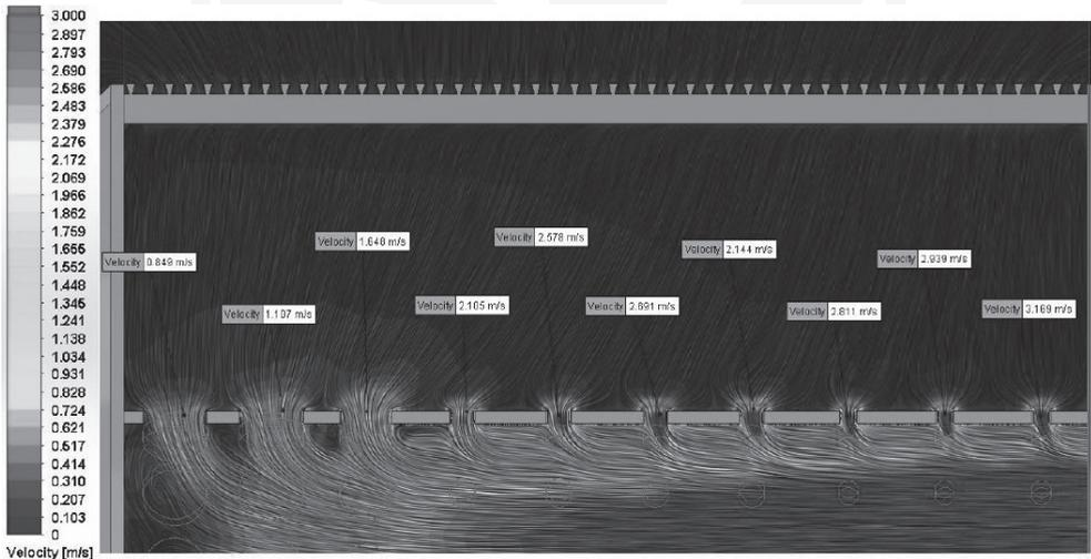
Fig. 5. The velocity distribution in the deflector's slots
