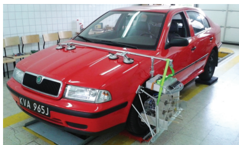
Fig. 2. An overview of a tested vehicle with the prototype measuring instrument mounted on the front left wheel
