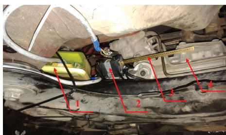
Fig. 3. Optical sensor of the linear displacements of the steering rack mounted in a test car: 1 – analogue-to-digital converter, 2 – sensor's housing, 3 – movable strip of a sensor, 4 – rack and pinion housing
