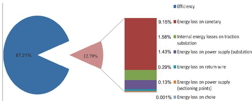
Fig. 7. Percentage breakdown of consumption of drawn energy in the analyzed case
