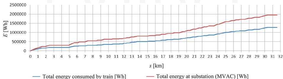
Fig. 6. Curves illustrating energy consumption recorded by the meters during the passage of the train
