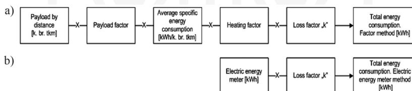
Fig. 1. Methods for calculating electrical energy consumption in PKP Energetyka S.A.: a) index method, b) meter-based method
