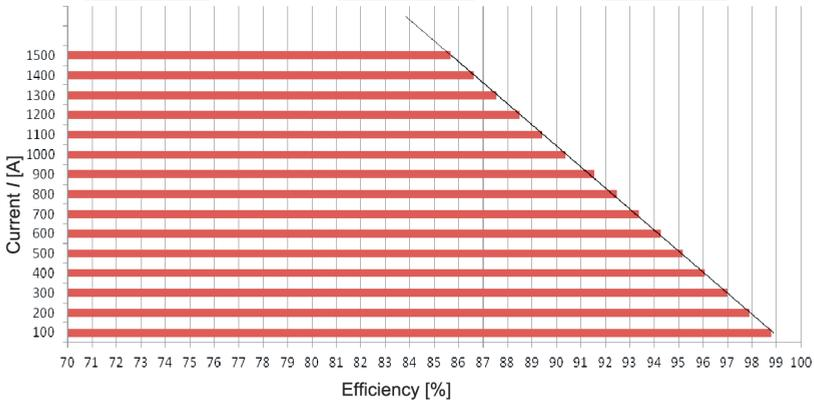
Fig. 12. Efficiency of the power supply system depending on the value of constant load current
