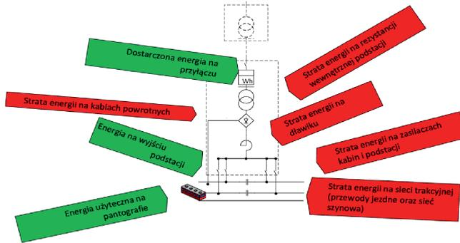
Fig. 2. Energy losses in the power supply system of an electrical traction vehicle
