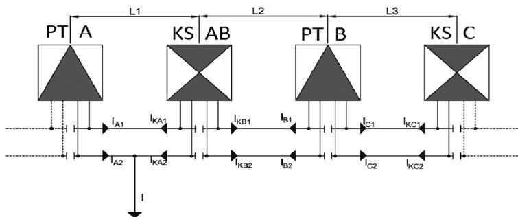
Fig. 3. Simplified model of the power supply system of a railway line section
