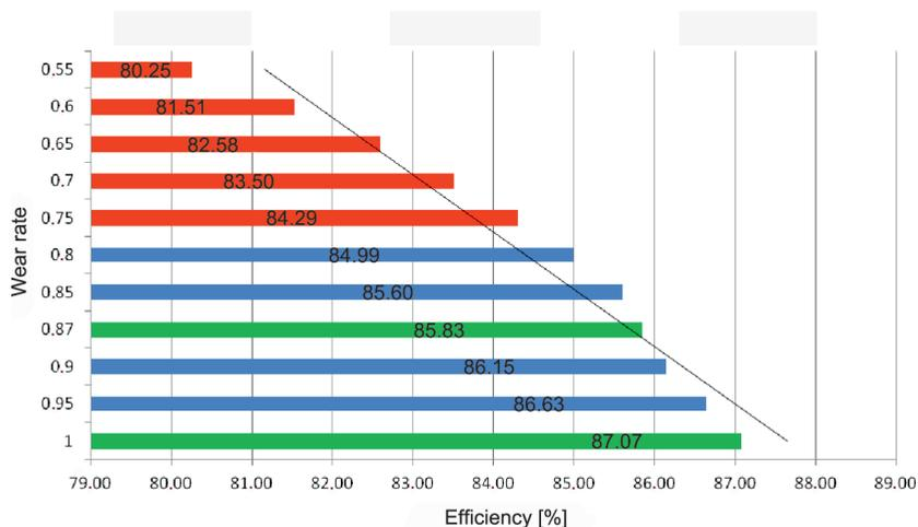
Fig. 9. Efficiency of the power supply system depending on the extent of wear and tear of contact wires
