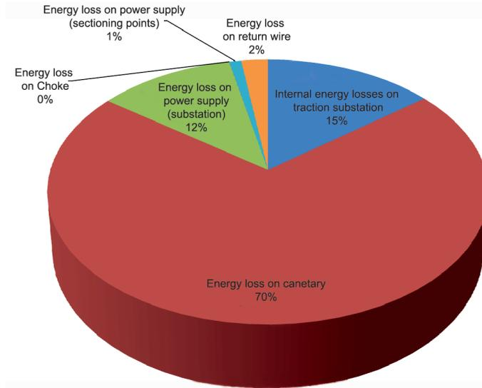
Fig. 8. Average balance of energy losses in the power supply system
