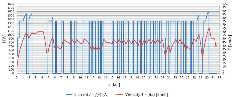
Fig. 5. Results of a theoretical passage for a selected case
