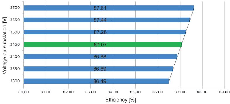
Fig. 11. Efficiency of the power supply system as a function of off-load voltage at the substation
