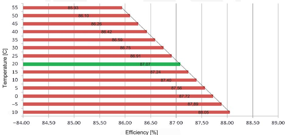
Fig. 10. Efficiency of the power supply system as a function of conductor temperature
