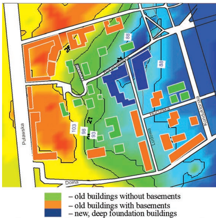
Fig. 12. Situational plan – upper model surface generated in HydroGeoBuilder software, with introduced localization of buildings and roads; levels are given in m a.s.l.
