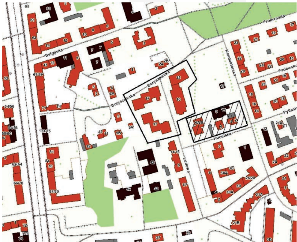
Fig. 9. The new deep foundation buildings are surrounded by a black line. The striped field depicts the area of existing buildings whose basements are damp [map source: geoportal.gov.pl]
