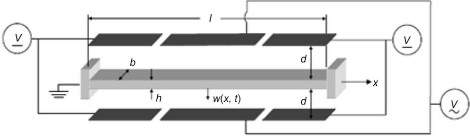
Fig. 2. Parametrically excited microbeam actuated by electric field [4]. The letter  $x$  in this figure denotes a coordinate of the cross-section of the beam
