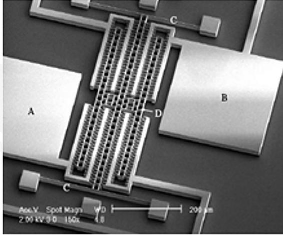
Fig. 1. Parametrically excited MEMS oscillator – electron microscope image [1]
