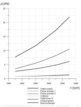
Fig. 5. Flow resistance in each component of the outlet system [3]
