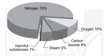
Fig. 6. Sample composition of exhaust gases from self-ignition engines [6]
