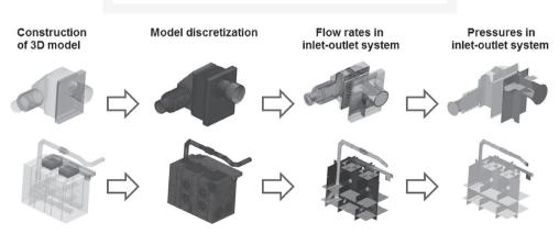
Fig. 4. Simulation tests of inlet-outlet system with use of CFD software programme [3]
