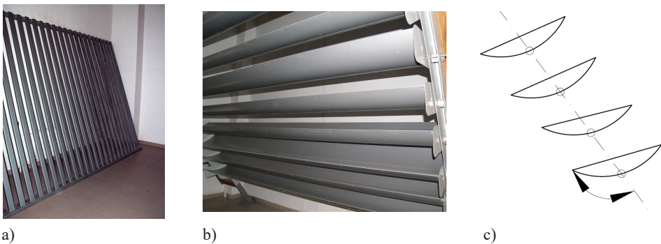
Fig. 2. Elements at the inlet to the wind tunnel: diagonal openwork shield (a), guide vanes (b), angle of the guide vane inclination (c)
