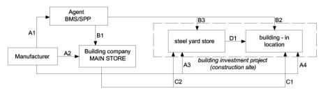
Fig. 1. Organisation of logistic chains for reinforcing steel deliveries to its building-in location
