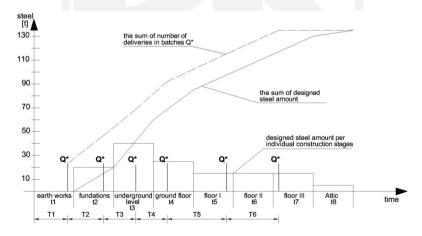
Fig. 2. Diagram showing steel demand for a building of improved conventional structure with trajectories of calculated material deliveries, Ti – intervals between deliveries, ti – reinforcement making durations at individual construction stages (Own study)
