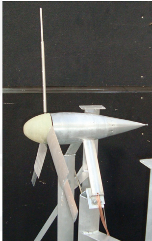
Fig. 12. Photograph of wind turbine model with stepped blades mounted on the instrumented hub
