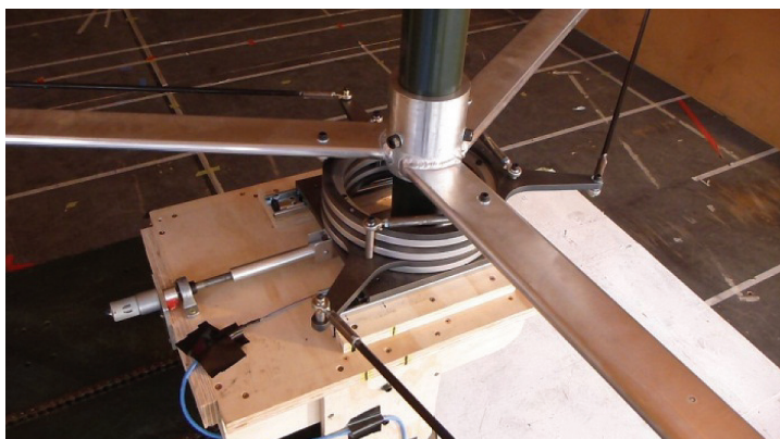
Fig. 17. Voith Schneider linkage system used to alter the angle of attack of the blades during each rotation
