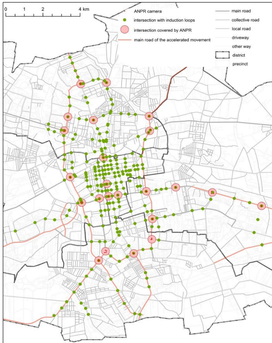
Fig. 1. The deployment of RTCS inductive loops and ANPR cameras in Lodz.
