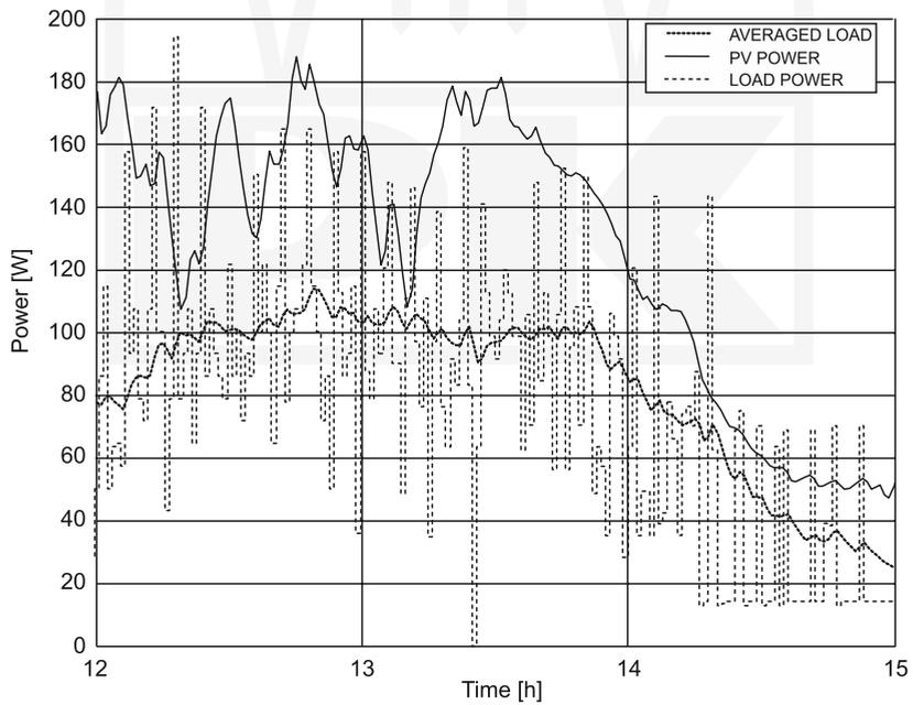
Fig. 7. Pulsed character of load power
