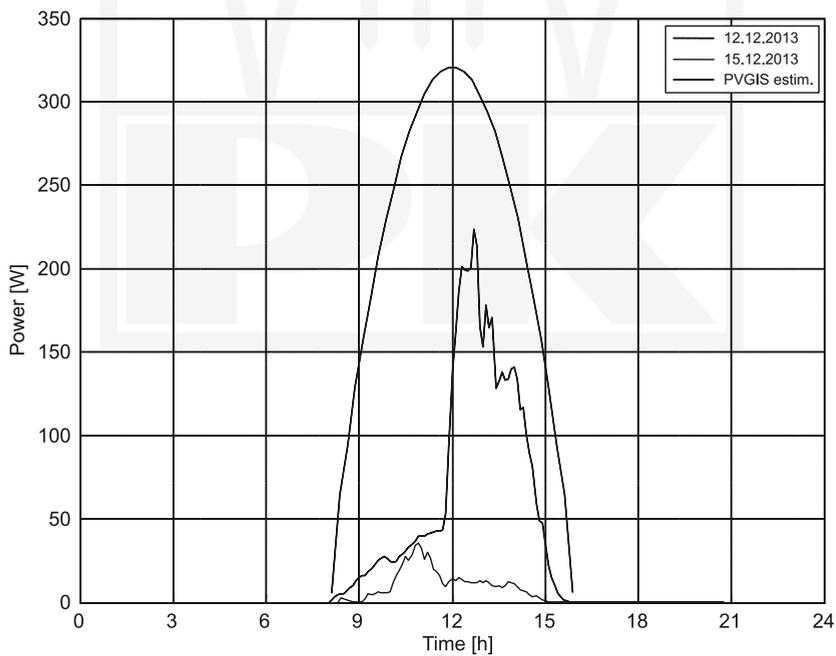
Fig. 5. Comparison of generated power for sample sunny and cloudy days (winter)
