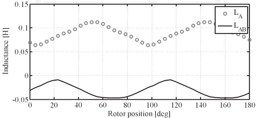
Fig. 7. FEM calculated inductances for nominal current
