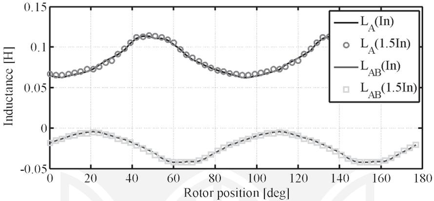
Fig. 6. Measured inductances for different current values
