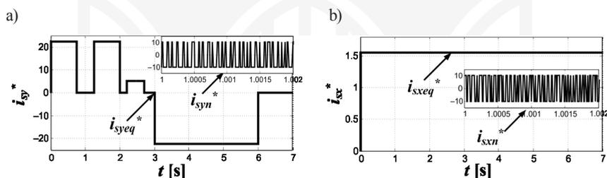
Fig. 5. Simulation results: a) the output signal  $i_{sy}^*$  from Sliding-Mode Controller of motor angular speed and b) the output signal  $i_{sx}^*$  from Sliding-Mode Controller of magnitude of the rotor flux vector
