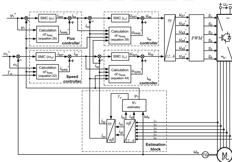
Fig. 1. Sliding-Mode DFOC of six-phase squirrel-cage induction motor
