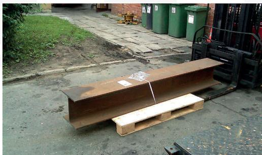
Fig. 10. Product from a steel mill prepared for installation in the existing suspended transport system – wide-flange HEA 320 I-section (photo. from the author’s archive)
