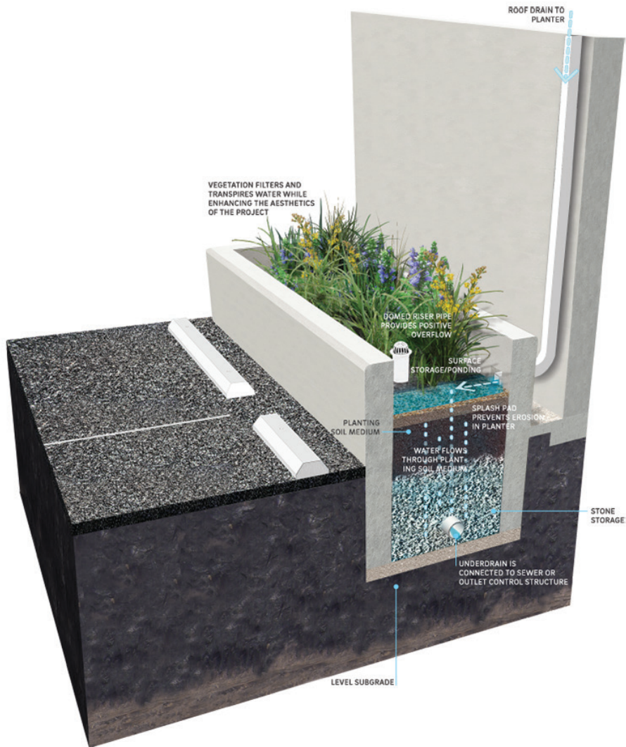
Fig. 10. Flow-Through Planter Box with Typical Features (source: [18])
