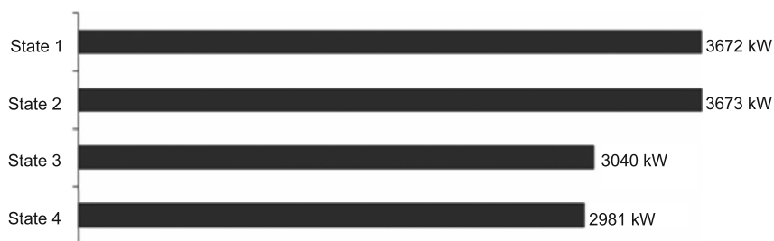
Fig. 7. Active power in different arc work states
