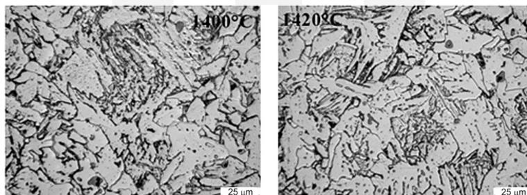
Fig. 13. Microstructure of samples deformed at 1400°C and 1420°C. Tool velocity 100 mm/s.
