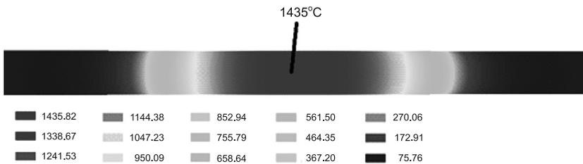
Fig. 7. Temperature distribution for simulation of heating to 1400°C – whole sample
