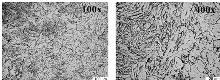
Fig. 12. Microstructure of sample deformed at 1400°C with tool velocity of 1 mm/s
