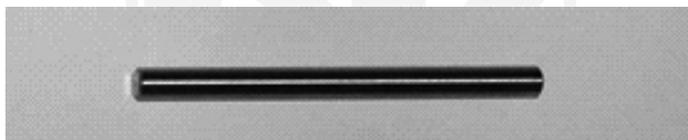
Fig. 1. Sample (6 × 82 mm) used to determine the NST temperature on the Gleeble 3800 simulator
