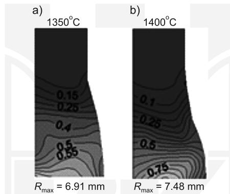
Fig. 10. The deformation intensity for high speed experiment (100 mm/s) – quarter of the sample ( $R_0 = 5$  mm)
