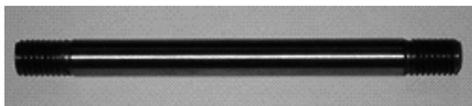
Fig. 2. Sample (10 × 125 mm) used to determine high-temperature characteristics of materials on the Gleeble 3800 simulator
