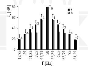
Fig. 5. Spectrum of phase stator currents for: a) four-stroke internal combustion engine, b) four-stroke internal combustion engine with doubled number of cylinders
