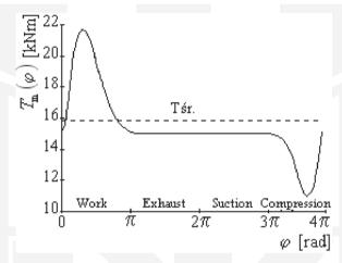
Fig. 1. The torque of the four-stroke internal combustion engine [2]
