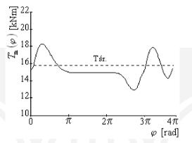
Fig. 4. Mechanical torque of the four-stroke internal combustion engine with double the number of the cylinders
