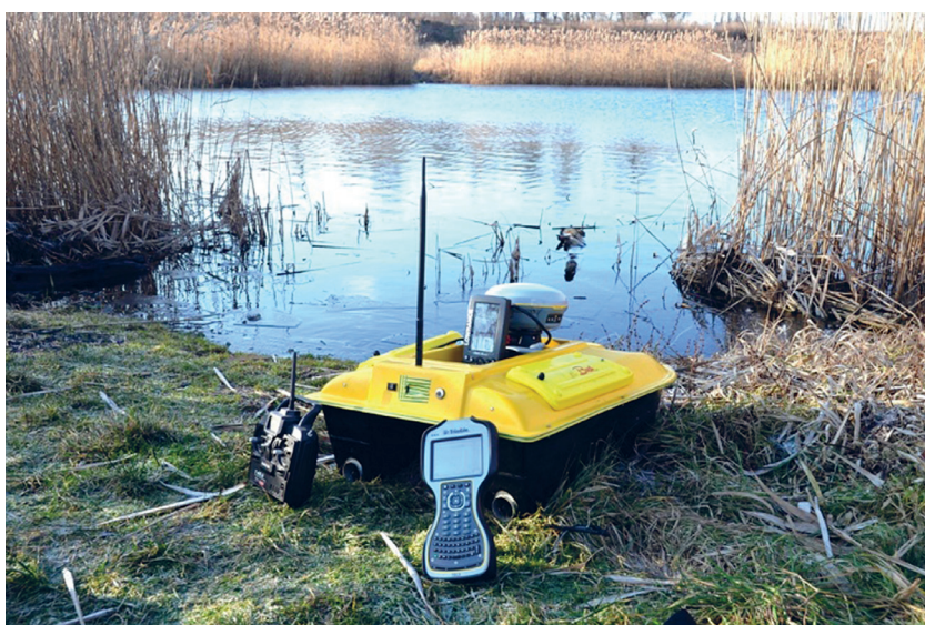
Fig. 7. The view of the measurement set: hydro-drone Smart-Sonar-Boat and GPS Trimble (aerial R8s + controller TSC3) during bathymetric measurements of the difficult-to-access part of the Bagry Reservoir. (Photo: D. Madusiok.)
