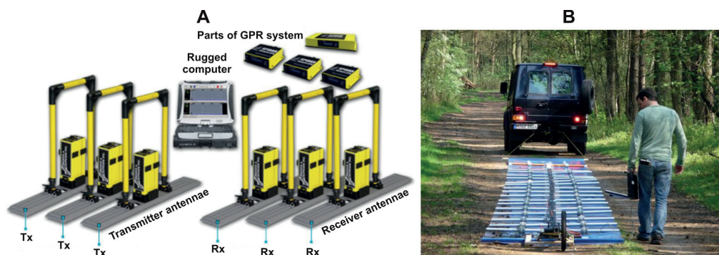
Fig. 3. Fig. 3. A) elements of a multichannel GPR system [37], B) terrain surveys with the use of GPR land streamer [39]
