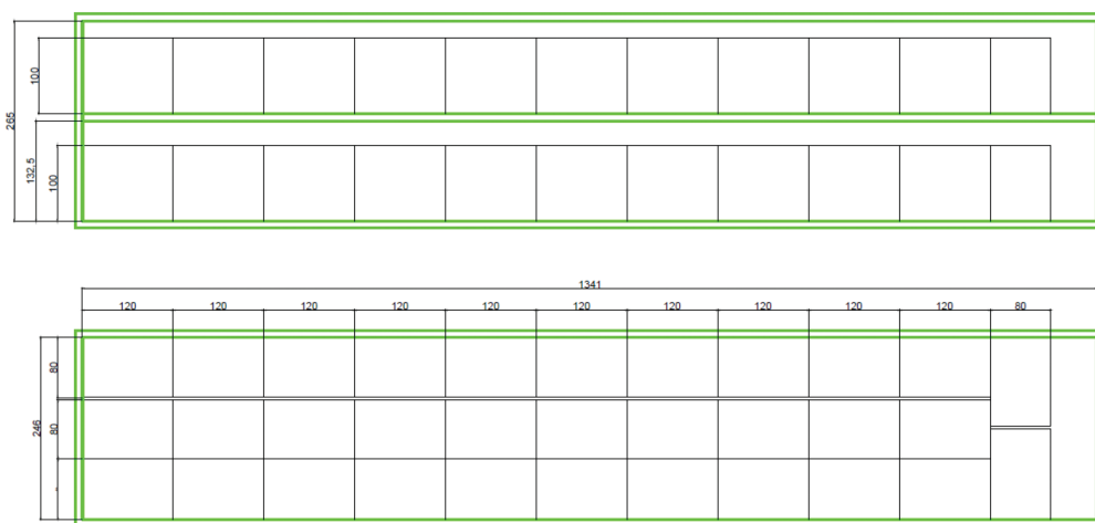
Fig. 19. [11] Example of pallet distribution in a refrigerated semi-trailer with a double-deck loading system
