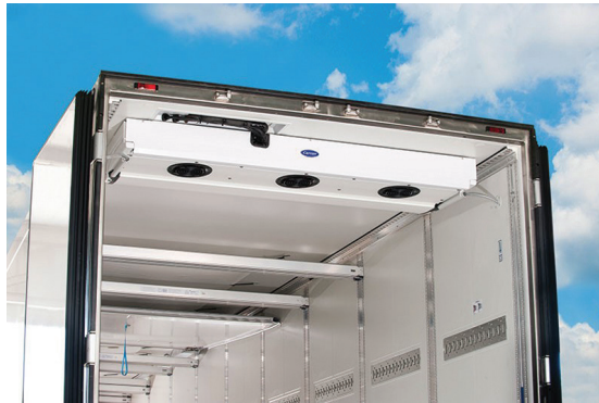
Fig. 8. Technical solutions (vertical bars) of load protection in refrigerated trailer Krone Cool Liner with ATD double-deck with Thermo King SLX 300
