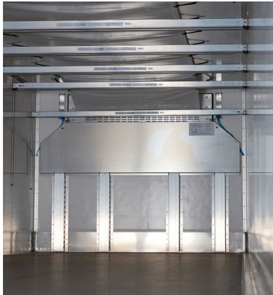
Fig. 7. ATD system – ATD loading beams with big loading capacity
