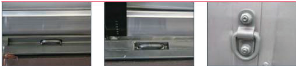
Fig. 16. Load securing fitting in the front wall, in accordance with EN 12640
