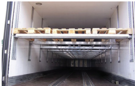
Fig. 9. Vertical and horizontal tracks securing cargo in side walls
