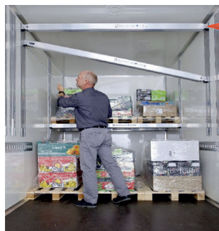
Fig. 6. ATD double-deck system consists of two elements: loading ATD beam and vertical airline tracks
