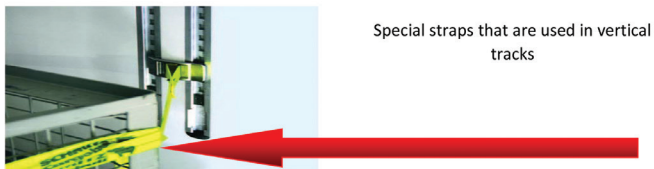
Fig. 3. System of load securing tracks on side walls; vertical and horizontal rods
