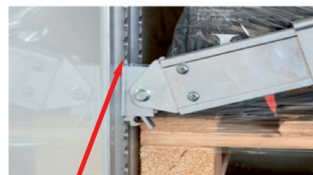
Fig. 6. ATD double-deck system consists of two elements: loading ATD beam and vertical airline tracks
