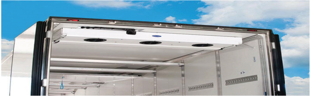
Fig. 10. Insulated roof filled with polyurethane foam, covered with steel sheet (up to 40 mm)
