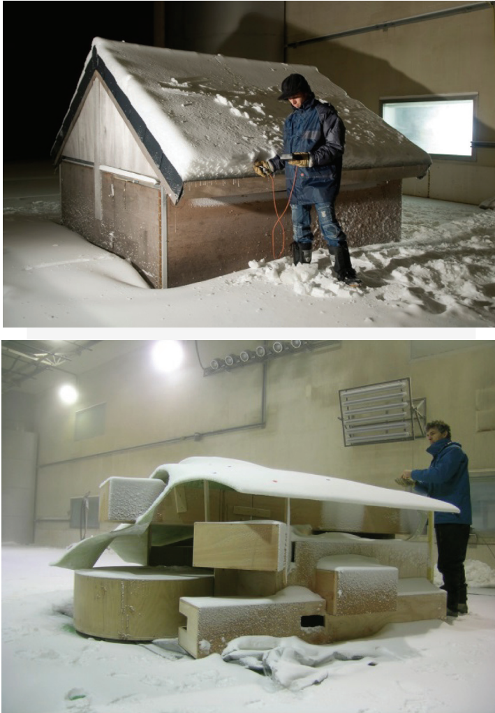
Fig. 4. Testing snow accumulation in the climatic wind tunnel at full scale (top) and reduced scale (bottom)
