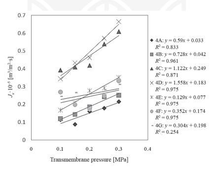
Fig. 12. The dependence of volumetric deionized water flux on pressure for membranes 4A to 4G
