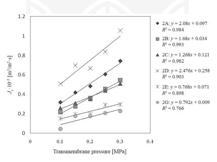
Fig. 6. The dependence of volumetric deionized water flux on pressure for membranes 2A to 2E, 2G
