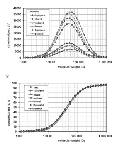
Fig. 13. Dextran molecular weight distribution curves in the feed and the permeate, obtained from the tests of membranes 4A-4G: a) correlation of the chromatogram height and dextran molecular weight, b) correlation between the cumulative share of dextran molecules and their molecular weight
