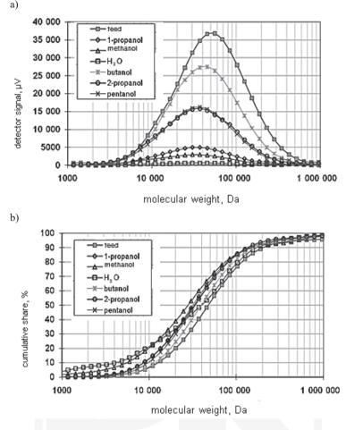
Fig. 4. Dextran molecular weight distribution curves in the feed and the permeates originating from the tests of membranes 1A to 1G (pure cellulose, gelled in various non solvents b) cumulative share of dextran molecules with the given weight
