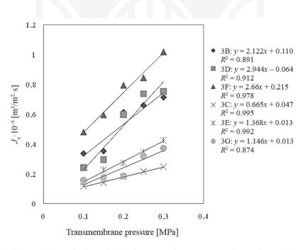
Fig. 9. The dependence of volumetric deionized water flux on pressure for membranes 3B to 3G
