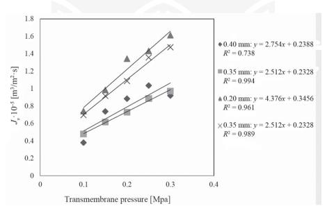
Fig. 2. The dependence of volumetric deionized water flux on pressure for cellulose membranes 0.20–0.40 mm thick
