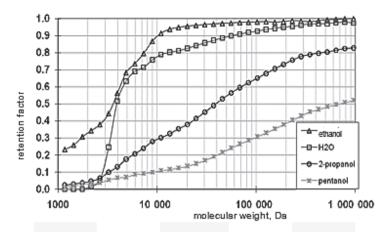
Fig. 11. Relation between the retention factor and dextran molecular weight, as determined for membranes 3B-3G
