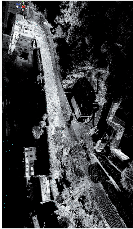
III. 4. Survey campaign using two laser scanners, in the entire accessible perimeter made so eliminating the vegetation (cloud of points a screen shots)
