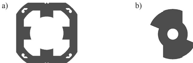
Fig. 1. Geometry of the 4/2 SRM: (a) stator, (b) rotor
