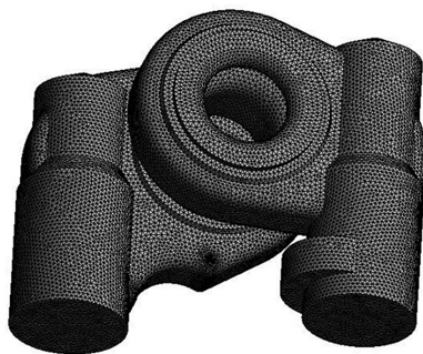
Fig. 4. Mesh of PA flow path
