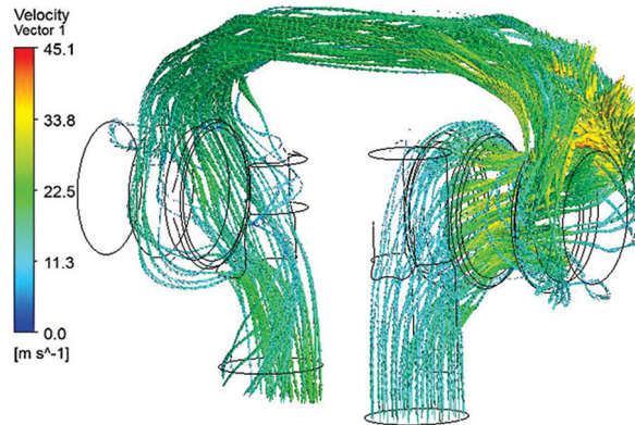
Fig. 9. Fluid velocity vectors along the stream lines for BT flow path
