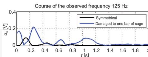
Fig. 12. Change of the observed frequency 125 Hz
