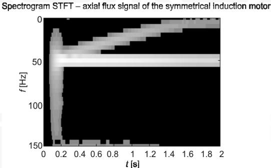
Fig. 10. Spectrogram STFT – axial flux signal of the symmetrical induction motor
