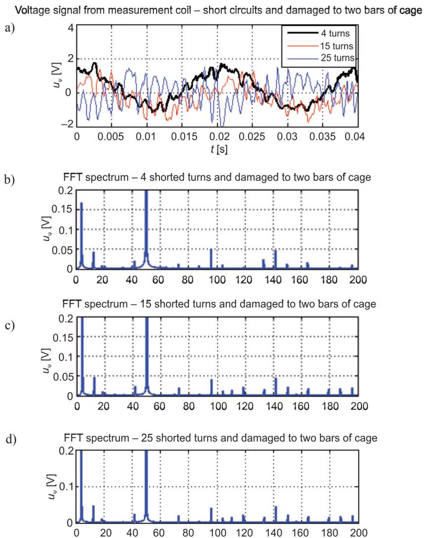
Fig. 8. Short circuits and two bars of cage damaged: a) voltage signal from measurement coil, b), c), d) FFT spectrum – shorted turns and two bars of cage damaged
