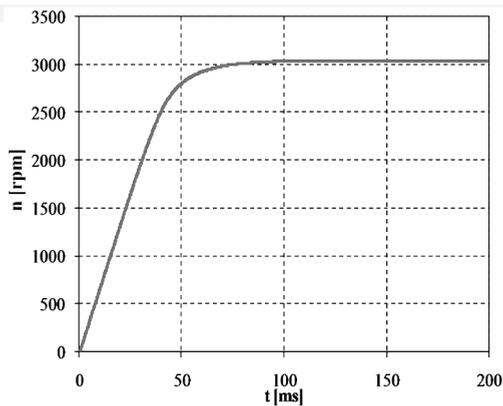
Fig. 16. Rotational speed at the motor start-up
